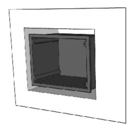
**2.** Use the 4 screws to attach the reduction frame to the recess box with the white dot facing upwards. Before tightening the screws, rotate the frame to align it in a horizontal position. Then tighten the screws.
