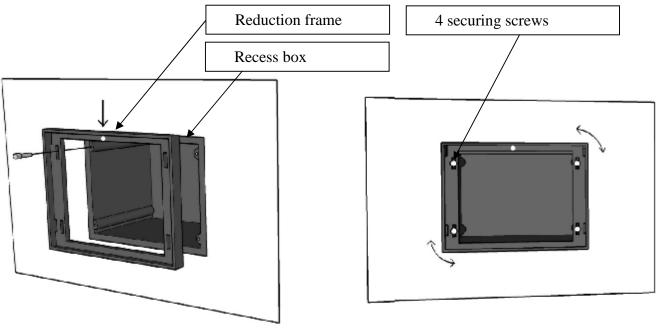
**3.** Before installation of the control unit, connect all cables, including the temperature sensor. Mount the control unit with the front panel on the frame by placing the hooks into the holes and pulling downward.
