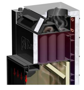
is very important for a comfortable cleaning, because it always comes to a settling of products of combustion on the inner walls of the pipes. The smaller the inside diameter of the pipes, the quicker their section becomes smaller during heating due to the settling of particles contained in the smoke, and the more difficult and more frequent their cleaning is.
