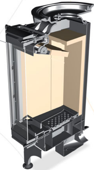
KV 025 FP/REDUCTION section
