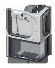
1- When the door of the combustion chamber is closed, the convective RMT flaps are opened at 100 %. Thanks to that air can flow and the travels of the extending door mechanism can be cooled down.
