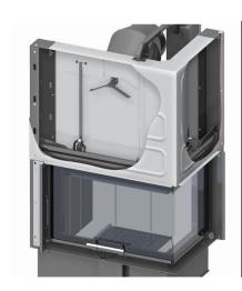
3- When the door is about 3 cm thrown up, the convective ROMOTOP® flaps are already totally closed and this prevents the smoke to get into the enclosure of the insert.
